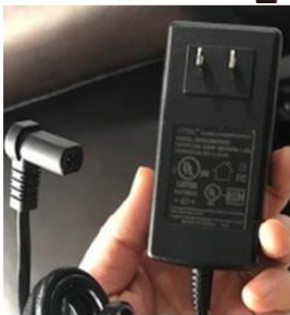
Low voltage Transformer wall plug In for power – 24Volt
